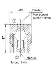
If the valve is used as reverse check, the user needs to change the position of o-ring
