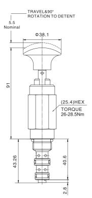
During installation,pilot drill Φ 12.7mm is required with min depth of 46mm. Orifice disc could not be used with this valve Unit=Millimeters
